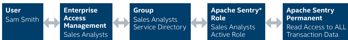
Figure 4. We use a role-based access control model that combines Apache Sentry* roles and directory service groups to grant permissions for Hive* and Impala* objects.
